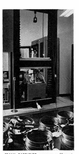
FRANK BATCHELOR prepares a filament wound specimen for static testing. The universal test machine will load the hoop in compression and the resulting measurements will indicate the material's strength. In the foreground are more samples awaiting test.
